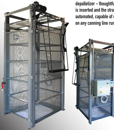
The Can-i-Bus is Ska Fab's original, small footprint, semi-automated can depalletizer - thoughtfully designed to fit your space and budget. Once a pallet is inserted and the straps and tier frame are removed, the Can-i-Bus is fully automated, capable of depalletizing multiple sized packages of various materials on any canning line running at 25 - 600 CPM with proper conveyance.
